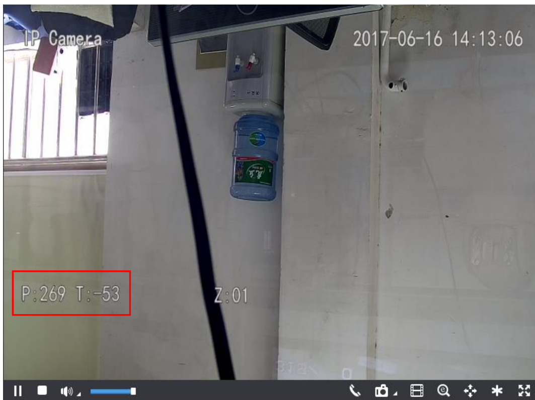
Picture 4-18 Azimuth Positioning- according to PT position
